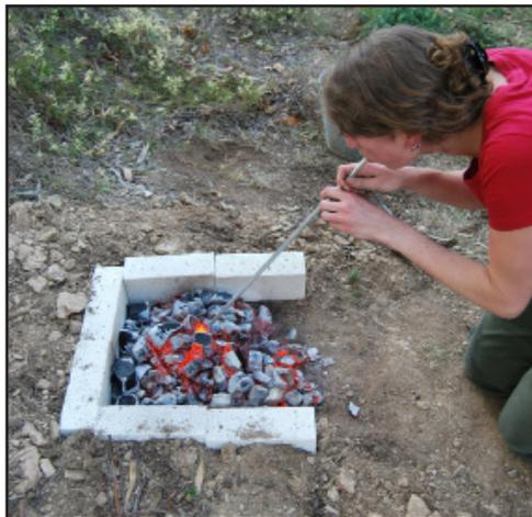
Figure 8: Annealing a billet in the hearth with a blow pipe (photo by L. Nguyen-hoan).
