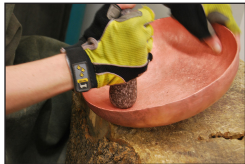
Figure 9: Sinking a vessel with a pestle into a hollow carved into a wooden stump (photo by L. Nguyen-hoan).
