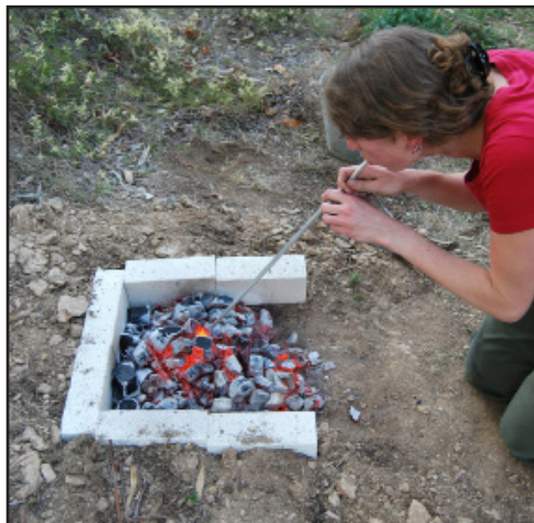
Figure 8: Annealing a billet in the hearth with a blow pipe (photo by L. Nguyen-hoan).
